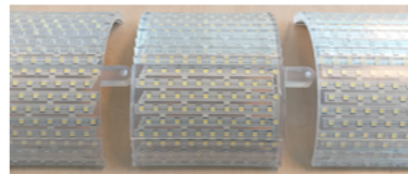
"FlexEnable LED matrices, overmoulded by PROMOLDING with a light-directional lens system designed by SnellOptics".
