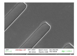
"ADAMA innovations IIL structured grating, replicated by PROMOLDING with their injection moulding machines".
