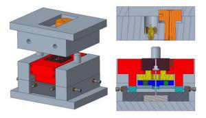
"Final concept of the mechatronic device for in-mould alignment and compensation of geometric tolerances".
