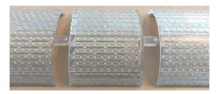
"FlexEnable LED matrixes, overmoulded by PROMOLDING with a lightdirectional lens system designed by SnellOptics".
