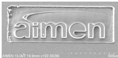
"AIMEN logo replicated by injection moulding from a photopolymerized hard resin insert".
