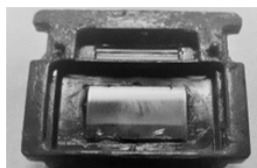
"Injected OEH with black, opaque frame and transparent optical elements. The top is a cylindrical lens".
