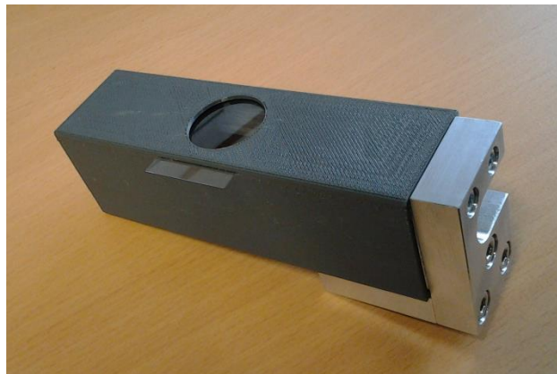
Figure 5 Single point probe head of an OCT setup. Length is around 15 cm.
