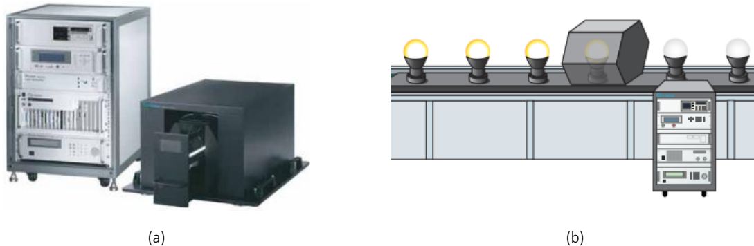
Figure 22 (a) View of the online test of photonic components for lighting, model 58158-SC developed by Chroma A.T.E. This model offers measurements of the total luminous flux emitted, and priority parameters in the components applied to lighting such as the correlated color temperature and the chromatic reproduction index. (b) Illustration where model 58158-SC operating line is indicated
