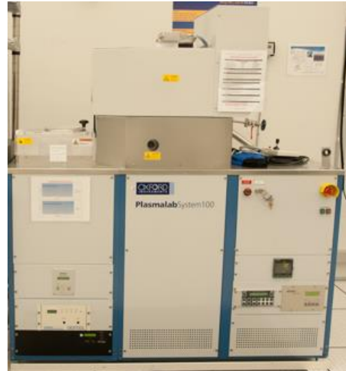
Figure 11. Plasmalab 100 ICP 180 etching tool used for our process.
