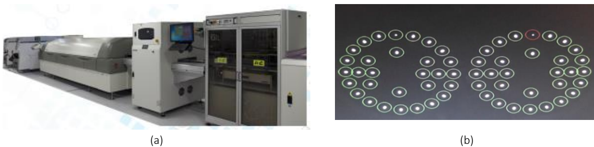
Figure 21 (a) Fully automated in-line test system for testing LED light engines developed by ATE Solutions. This system of in-line validation of photonic components evaluates the absence or if the photonic component does not emit enough luminous flux. (b) Appearance of the record that assesses the ATE Solutions system, where it is indicated by a red circle that the photonic component does not emit enough luminous flux.
