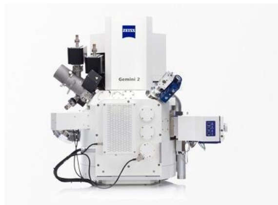
Figure 10: The Carl ZEISS Focused Ion Beam Scanning Electron Microscopes (FIB-SEMs) used for the nanopatterning process.
